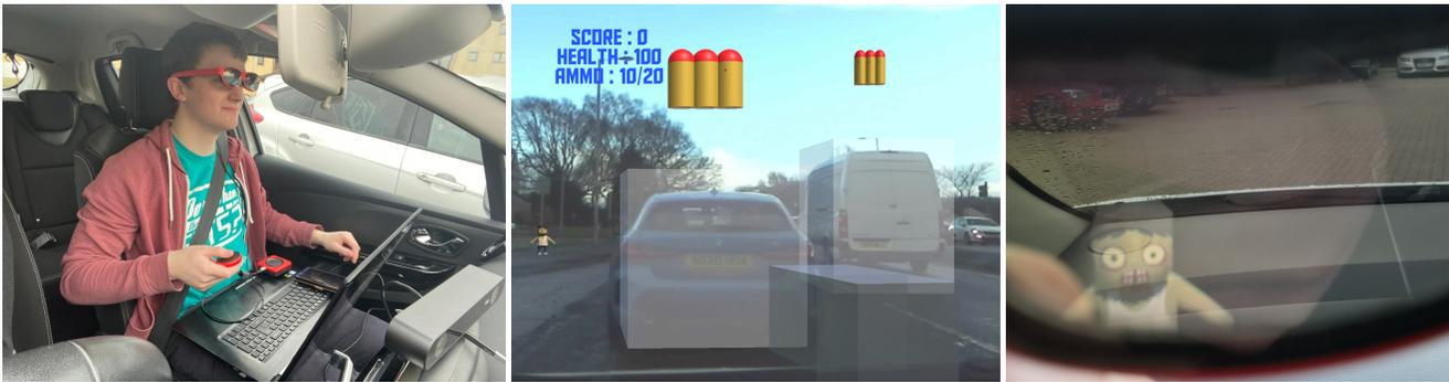
**Figure 2: Game Prototype Two. Hardware setup, with ZED 2 on dashboard, AR glasses, server laptop and controller puck (L). Composite of AR view and captured video of journey illustrating experience (M). Zombie captured through the AR headset lens (R).**
