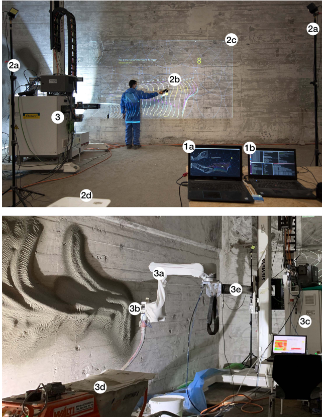
Figure 6: User interaction-tracking system including visualization computer (1a), ROS master (1b), VIVE tracking system (2a), controller (2b), projection mapping (2c), projector (2d); Right: Robotic fabrication setup including UR10 robotic arm (3a), spray gun (3b), controller box (3c), pump (3d), external axis (3e).
