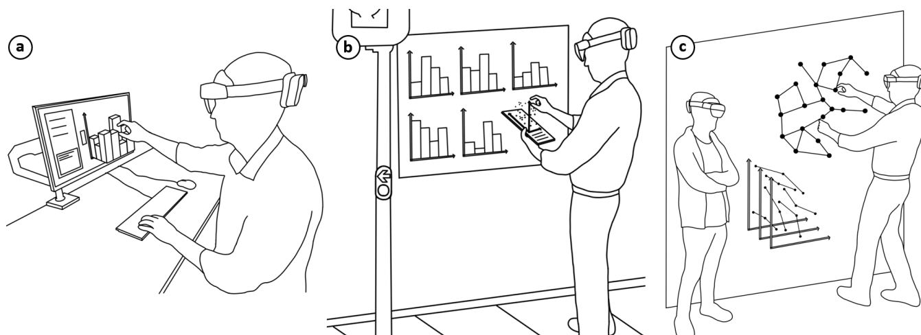
Figure 1: Conceptual future scenarios of 2D and 3D transformations and mixed-reality data visualisation. (a) A user at a desktop extrudes a 3D bar chart by grabbing and pulling from the monitor. (b) A remote worker on the side of a street extruding a 3D scatterplot from a tablet with a virtual surface aiding organisation of a faceted bar chart. (c) Two collaborators visualising data on a wall without the need for large high-resolution displays.
