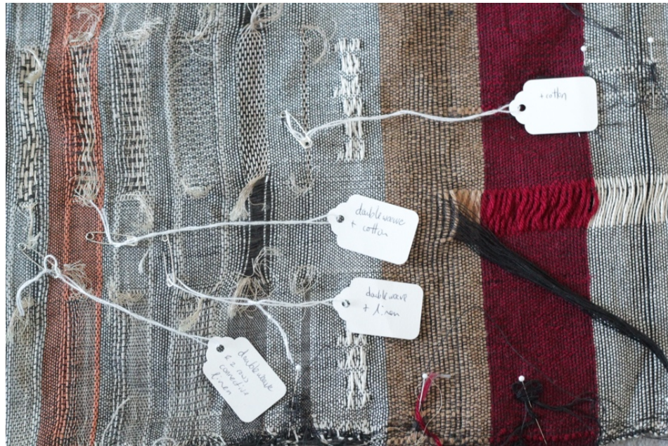
Figure 11: photograph of the labelled antenna sample before cutting and scanning (the observant reader may recognize some pins and knots from Figure 8).
