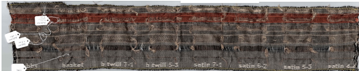
Figure 10: A scan (stitched together in photoshop) of woven antenna sample with labels and woven text indicating the difference between swatches
