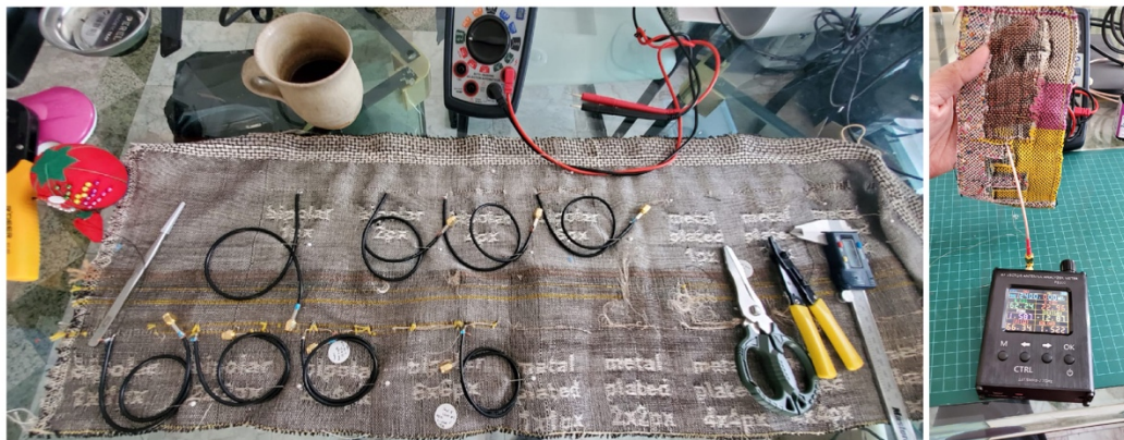
Figure 12: Henry's set up to test the antennas, including clippers, a multimeter, and coax cables that need to be attached to each sample, and testing an antenna sample with a vector antenna analyzer.
