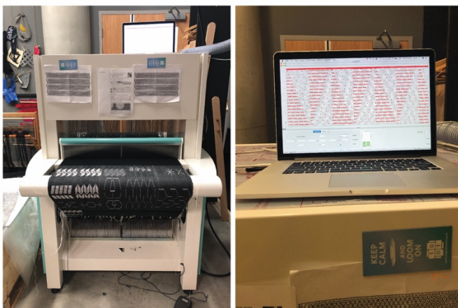
Figure 4: the loom with some first weaving samples and the MacBook pro with the TC2 software.
