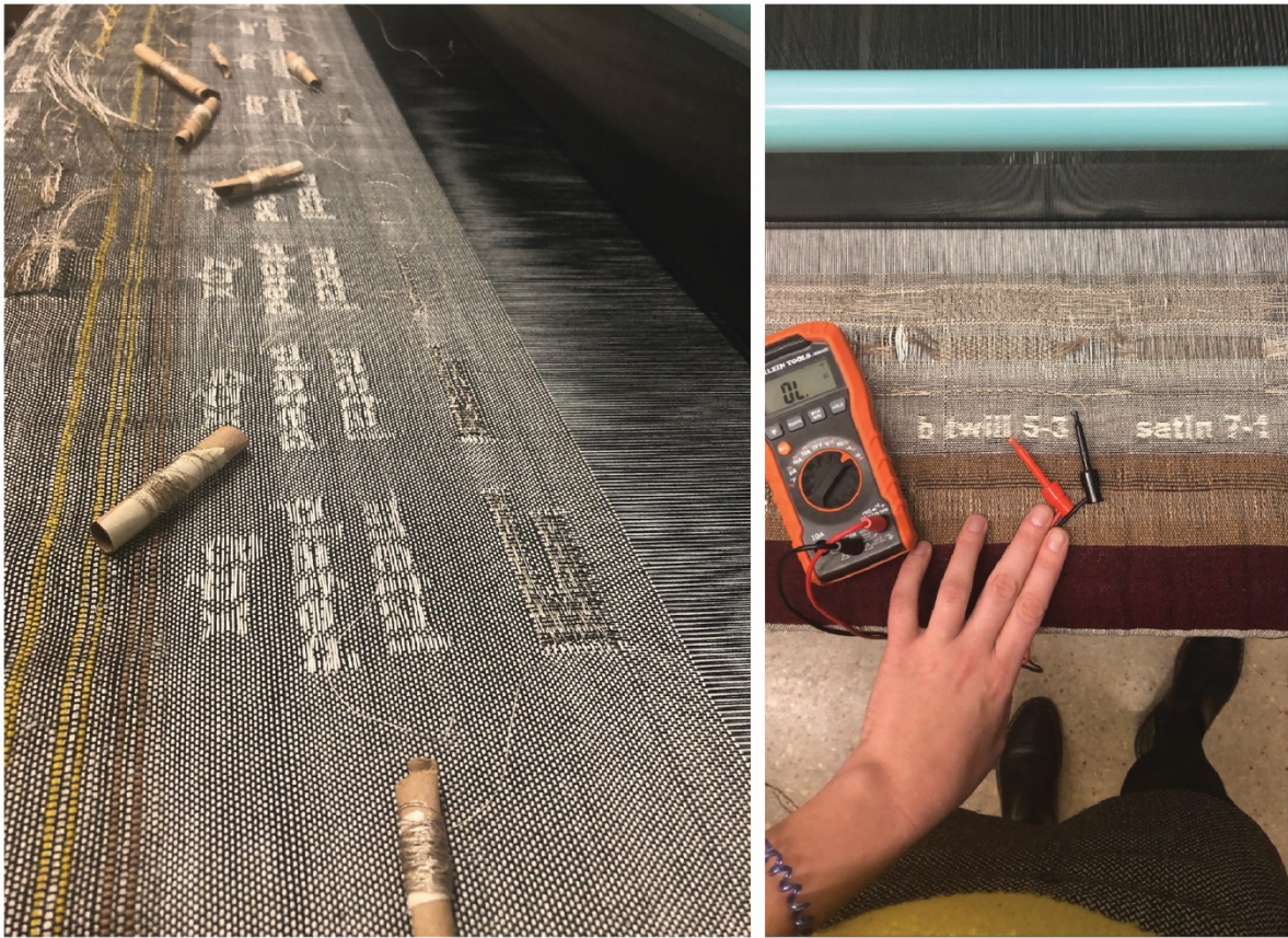
Figure 9: weaving with the conductive material on separate bobbins as additional weft and measuring connectivity with the multimeter
