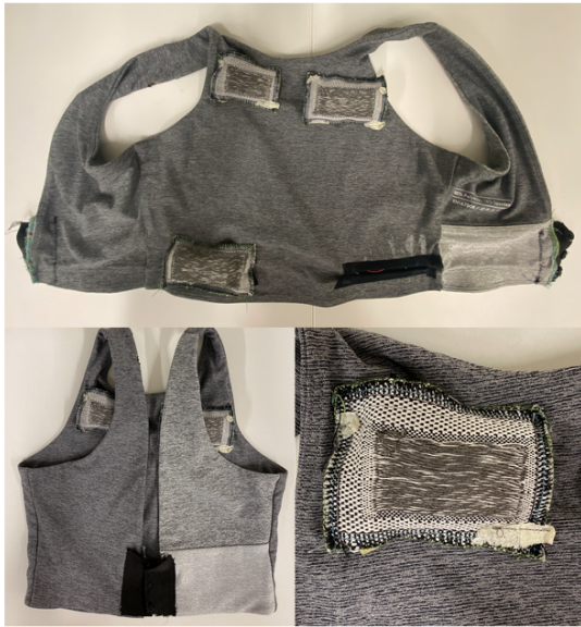
Figure 6: Final ARGONAUT garments with sensor, electronic, and closure mechanism integration.
