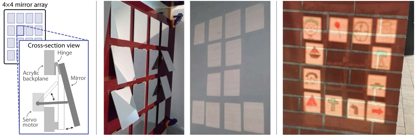
Figure 3: (a) SolarPix in operation. Left: a 4×4 array of mirrors is individually actuated to direct light either to a nearby surface (two rightmost images) or to a solar panel mounted above (the dark area just visible at the top of the centre left image). Centre: SolarPix provides light output by reflecting light ‘pixels’ in meaningful patterns. For example, the ‘T’ shape shown here is created by actuating four of the 16 mirrors to direct light away from the projection surface. Right: the device’s pixel mirrors can themselves be augmented with pictograms to add a further layer of output and meaning by combining both light patterns and sketched icons.
