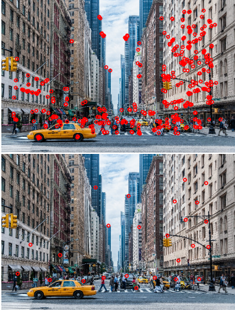
Figure 3: The figure above is the area represented by the direct calculation of ORB feature points. Obviously a large number of points are clustered on the same feature area. The bottom figure represents the ORB feature points after local clustering. It's apparent that the number of feature points is significantly reduced, and there will only be one ORB feature point in a local region.
