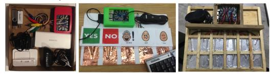
Fig. 1. The TalkBox prototyping platform, as a kit (Left), assembled as a communication board (Middle) and redesigned to be more robust with increased touch surfaces (Right).
