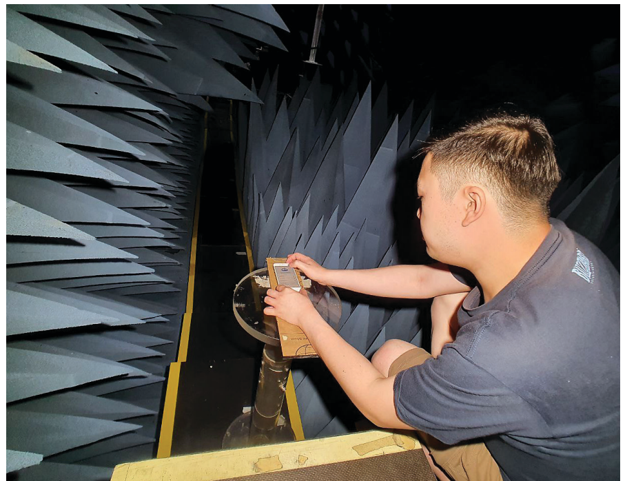
Figure 2, Performing characterization testing of handsets in an anechoic electromagnetic test chamber.
