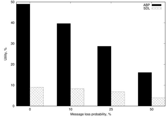
Fig. 5. Reliable Data Link. Message utility depending on message loss.
