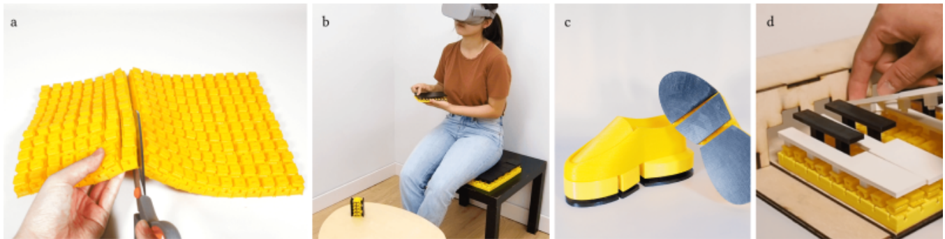
Figure 1: We propose a reconfigurable metamaterial that can be easily and repeatedly reconfigured by end users. We envision (a) that the generic material sheet can be purchased as larger sheets, and be cut and configured to opportunistically augment the elastic properties of objects. We show how this material can be applied to realize applications, such as (b) passive haptic props for VR, (c) custom shoe soles or (d) piano keys.
