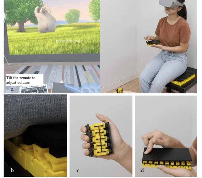
Figure 6: (a) The user is watching a VR movie with tactile props made from our material, including (b) a simulated sofa, (c) a pump to adjust the screen size, and (d) a remote control to adjust volume and playback speed. We use Oculus’ built-in hand tracking to track the hand motions when interacting with the passive props.
