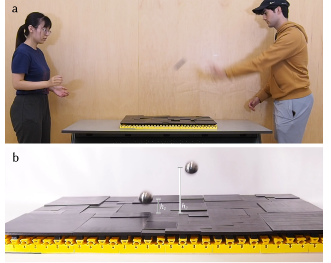
Figure 12: A ball game that combines pong and battleship. (a) Users throw a ball onto the material, but could previously configure (b) the local elasticity to make it difficult for their opponent to catch the ball. The map is concealed as the configuration layer looks identical from the top.
