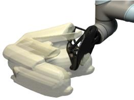
Fig. 7. In the robot’s reference frame, the swept volume of the bunny (shown in white) is the space occupied by the bunny throughout the trajectory. The complementary space is the *collision-free* space for topology optimization. The topology optimized gripper is shown in black.
