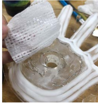
Figure 3.15 Hot wire is on the hand model to present the skin temperature
