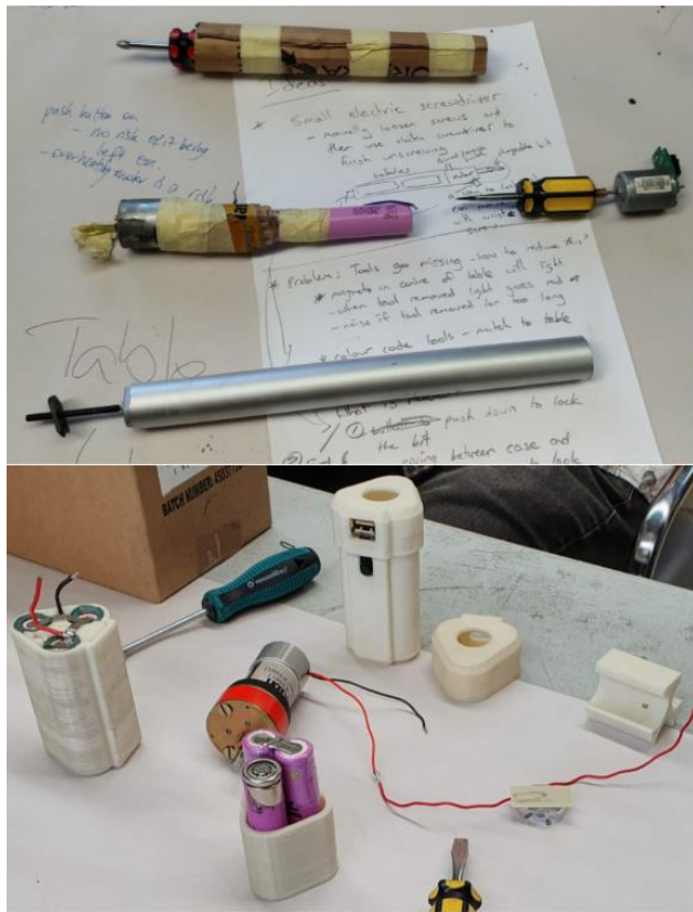
Figure 5. Screwdriver prototypes developed within the maker workshop. Top: Ergonomic prototypes (top, bottom), and motorized prototypes (both middle); and Bottom: different housing devices were explored using 3D printed material.
