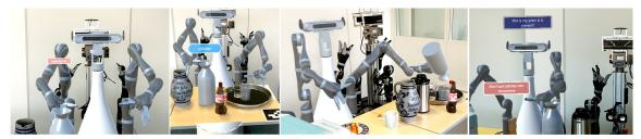
Fig. 3. Visualization of planning phases, from left to right: the user instructs the robot by speech; the robot shows its avatar and digital twins of real objects; the avatar executes the plan; the human gives feedback on the plan. Red boxes show the user's commands as detected by speech recognition.
