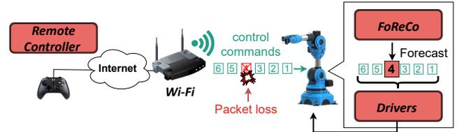
Figure 1: FoReCo forecasts/infers control commands lost in the wireless communication between the remote controller and the robotic arm.
