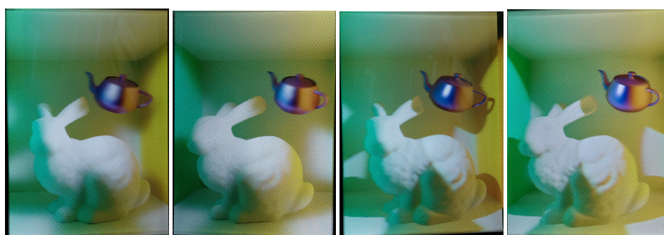
Figure 1: A scene with the “Stanford Bunny”, rendered in Tauray on an RTX 3090, shown from two viewpoints on the Looking Glass Portrait light field display. Left pair: denoised path tracing in ~50 ms. Right pair: DDISH-GI [Ikkala et al. 2021] in ~15 ms.
