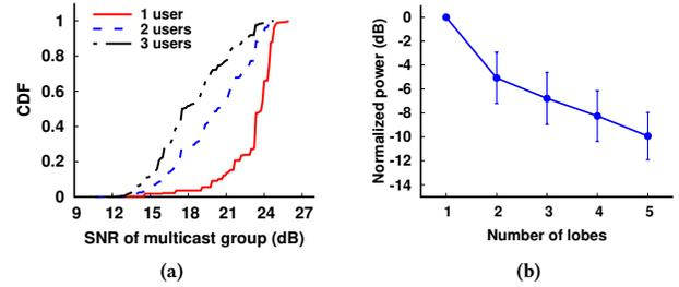
Fig. 11: (a) The default beams cannot support an efficient multicast (b) Reduction in peak power for multi-lobe beams
