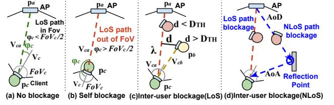
Fig. 7: M5's self and inter-user blockage prediction model
