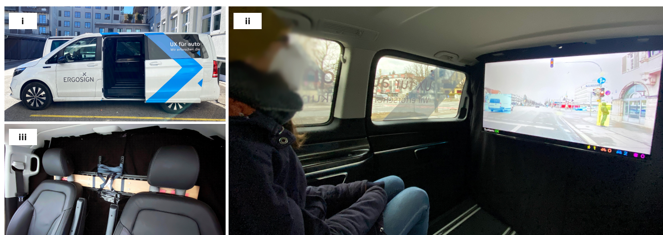
Figure 1: On-road wizard-of-oz prototyping in an electric minivan (i) with a TV mounted on the headrests of the front seats (iii) that displays a video stream from the vehicle's windshield with AR-based real-time object detection visualization (ii) provided by an embedded computing platform (Nvidia Jetson Nano).
