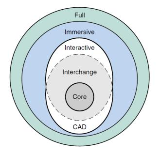
Figure 7: Profiles of X3D functionality permit componentized complexity in model sophistication and browser capabilities.
