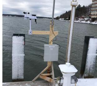
**Figure 3: Weather station outdoor sensor**
