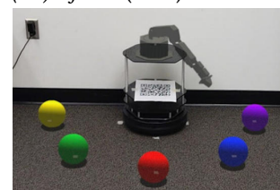
(d) Physical Robot with a virtual (AR) arm pointing to an virtual (AR) referent (V→V)
