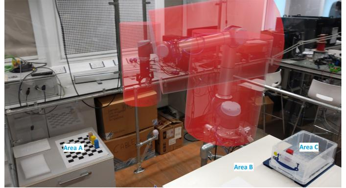
Figure 1: The robot arm picks up a wooden block from area A and moves it to area B, the middle of the table. The user then picks up the block from B and places it in the plastic container (area C).
