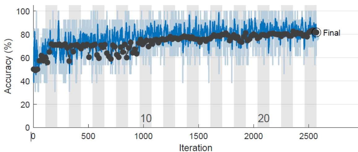
Figure 5: Changing of accuracy during the training process for normalised data input.
