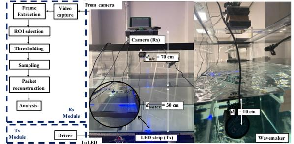
Figure 1: Experimental setup and decoding process of the proposed GS-based W2A OCC system.
