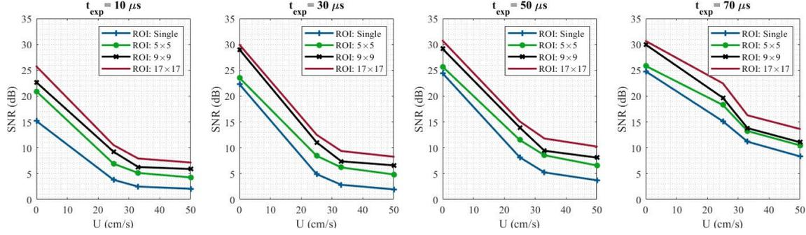
Figure 2: SNR for different wave speeds considering four different ROIs and camera exposure times of 10  $\mu$ s, 30  $\mu$ s, 50  $\mu$ s, and 70  $\mu$ s.
