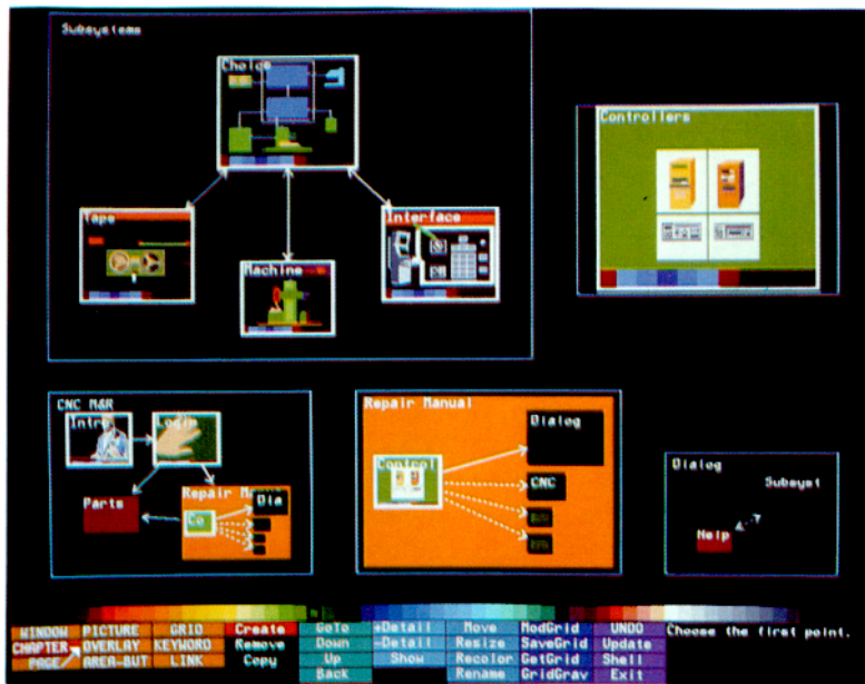
Fig. 4. A multiple window display in the document layout system. Each window contains a chapter or page. The author may traverse the document's structure independently in each window and make links between chapters and pages in different windows. Windows may be created, resized, and removed as needed.
