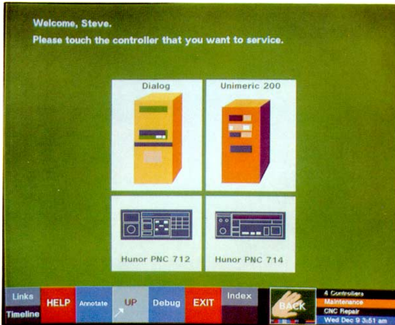
Fig. 5. A page from a document currently under development. The reader's selection of one of the four numerical controllers shown determines the page to be displayed next. All buttons (the controllers and the named rectangles along the bottom) were specified by the page's author. At the lower right, an automatically generated picture shows a miniature of the previous page (which serves as a back button), the names of the page, parent chapter and document, and the time.
