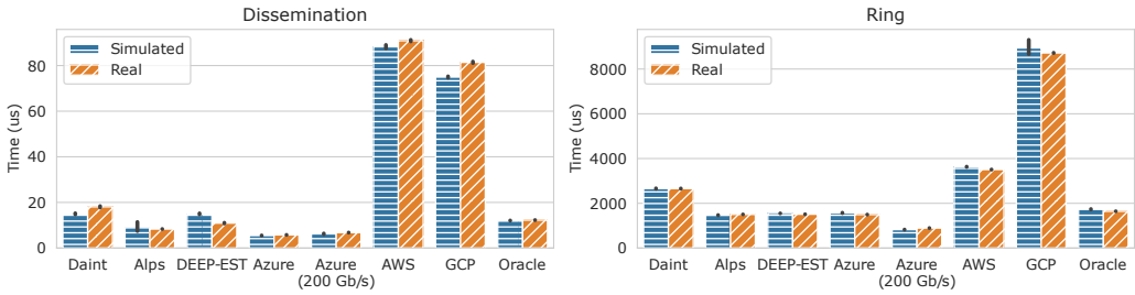
Fig. 19. Comparison between measured (on HPC instances) and simulated times for 16B on dissemination and 16MiB ring collectives on 8 nodes. Black vertical lines at the top of the boxes represent the 95% confidence interval.
