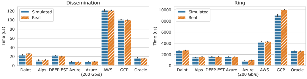
Fig. 13. Comparison between measured and simulated times (on HPC instances) for 16B dissemination and 16MiB ring collectives on 16 nodes. Vertical lines at the top of the boxes represent the 95% confidence interval.
