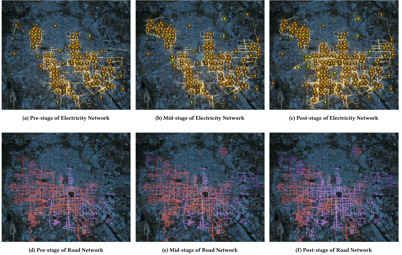
Figure 5: Process of finding vulnerable nodes in interdependent network
