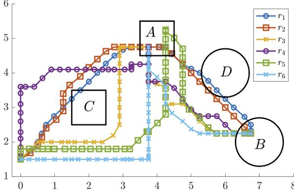
Fig. 2. The figure shows six potential robot trajectories  $r_1$ - $r_6$  and the four regions A, B, C, and D. The specification given in (2) is violated by  $r_1$  and satisfied by  $r_2$ - $r_6$ . It can be seen that  $r_2$  only marginally satisfies  $\phi$ , while  $r_3$ - $r_6$  satisfy  $\phi$  robustly.
