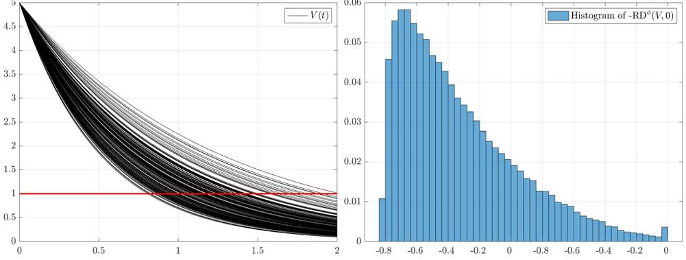
Fig. 4. Left: 200 realizations of the voltage  $V(t)$  over the capacitor of an RC circuit. Right: Histogram of the negative robustness degree  $-RD^\phi(V, 0)$  of the specification  $\phi := G_{[2, \infty)}(V \leq 1)$ .
