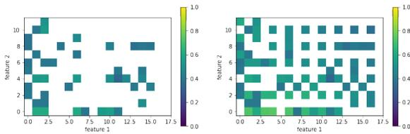
**Figure 3: A chosen focus-area (the right focus-area from Figure 1) before optimization (left) and after 57 additional observations in the focus-area (right). The gaps are filled with high performing points, the prediction model will now be significantly improved in this region.**
