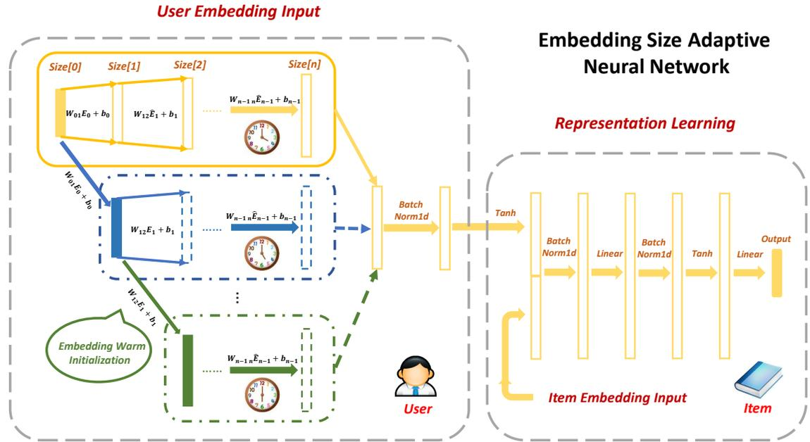
Figure 2: The illustration of embedding size adaptive neural network structure. Only the user embedding input is shown in detail above. The item embedding input structure is similar. Different colors indicate the model inference process at different timesteps. The dashed rectangles represent the tensors that do not participate in the current forward propagation. The hollow rectangles represent intermediate tensors that will not be saved after the neural network forward propagation.
