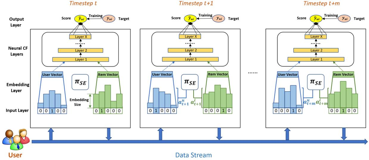
**Figure 1: Illustration of the dynamic embedding size search process. At each timestep, the embedding layer outputs embedding vectors with sizes determined by the  $\pi_{SE}$ . After transformation, they will be input into Neural CF layers for further inference.**
