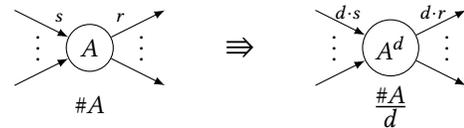
Figure 9. Firing reduction of actor  $A$  by divisor  $d$ .
