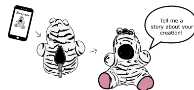
Figure 1: A graphic of the child-robot interaction. A mobile application running the voice interaction is inserted into a stuffed animal to create an interactive robotic object (IRO). The robot asks open-ended questions to support children in reflecting on their creative play through storytelling.
