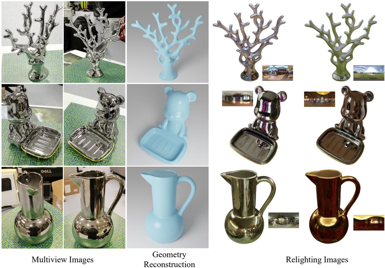
Fig. 1. **NeRO**. We present NeRO for reconstructing the geometry and the BRDF of reflective objects with strong reflective appearances. NeRO only requires multiview input images of the reflective object under an unknown illumination condition. The output of NeRO is a triangular mesh with material parameters, which can easily be used in rendering software for relighting and other applications.
