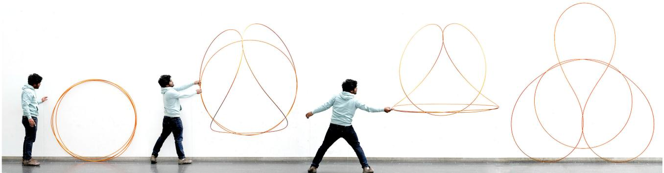
Fig. 1. A deployable structure built from a multistable elastic knot. The two center images show different orientations of the same 3D equilibrium state.
