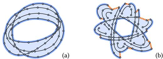
Fig. 6. For a sketch solely composed of closed strokes, its shape’s boundary is entirely supported by the input strokes (a). For a typical sketch with open strokes, however, its sketch shape boundary often includes additional connections (b, orange dashed lines).
