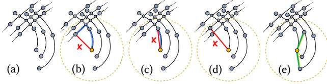
Fig. 9. Given the sampled input strokes (a), the Sketch Complex is composed of all segments between samples within  $\alpha$ -distance such that they are not already  $\alpha$ -connected (b,c) and do not intersect the sketch strokes (d). For the selected sample (e), the three allowed segments are in green, we only add the ones depicted in bold.
