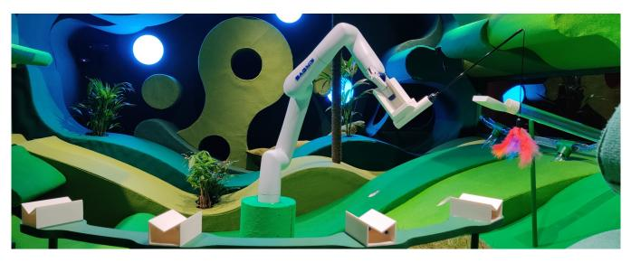
Figure 1: View of the environment with the Kinova robot at the centre and the end-effector attachment rack in the front.
