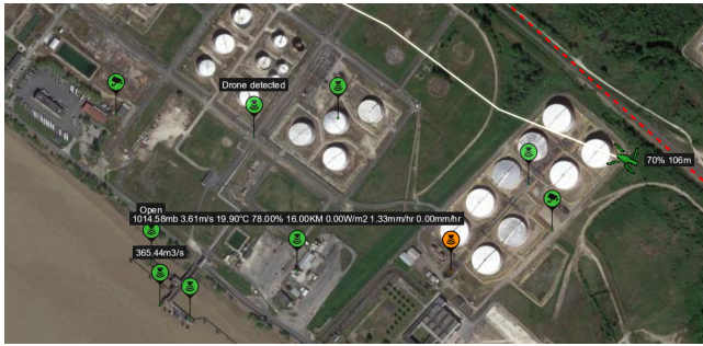
Figure 2: An instance of the PSA map view. The monitored values of each sensor are shown in real-time.
