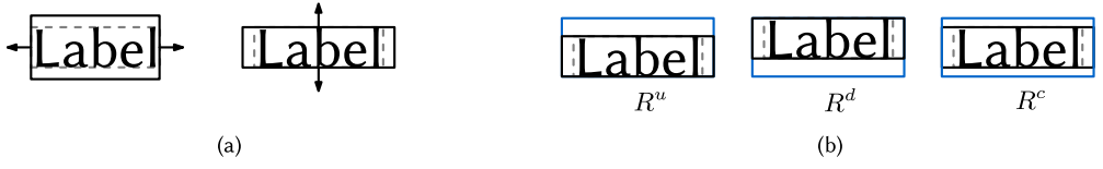
Fig. 8. Stretching R closer to the aspect ratio of the corresponding label l_R . (a) Stretching along major/minor axis depends on aspect ratio of R compared to l_R . (b) Three candidates for stretching: upwards, downwards, or both.
