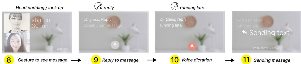
Fig. 15. Steps of sending a new message and Reply to a Message using Google Glass XE (Source: [30]). To Send a New Message , the user: (1) activates voice commands by saying 'OK GLASS'; (2) initiates the messaging process by saying 'SEND A MESSAGE TO'; (3) selects the recipient by saying their name (e.g., 'SARAH SMITH'); (4) starts voice dictation; (5) the system transcribes the user's utterances to text in real-time and stops transcription after a silence; (6) the system automatically sends the message unless the user explicitly cancels it using the touch interface; (7) the user sees the sent message as a notification while looking up, and it disappears when the user looks forward. To Reply to a Message , the user: (8) nods the head or looks up to see the received message; (9) initiates the replying process by saying 'REPLY'; (10) the system transcribes the user's utterances to text in real-time and stops transcription after a silence; (11) the system automatically sends the message unless the user explicitly cancels it using the touch interface.
