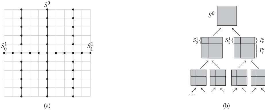
Fig. 1. (1(a)) The top three levels of nested dissection for an  $11^2$  mesh. The root separator  $S^0$  is a vertical 11-point line. The next level separators are  $S_0^1$  and  $S_1^1$ . The root separator corresponds to the top-level front in (b), and similarly for the next level down in the assembly/frontal tree. Note that the fronts in (b) typically get smaller lower in the tree.
