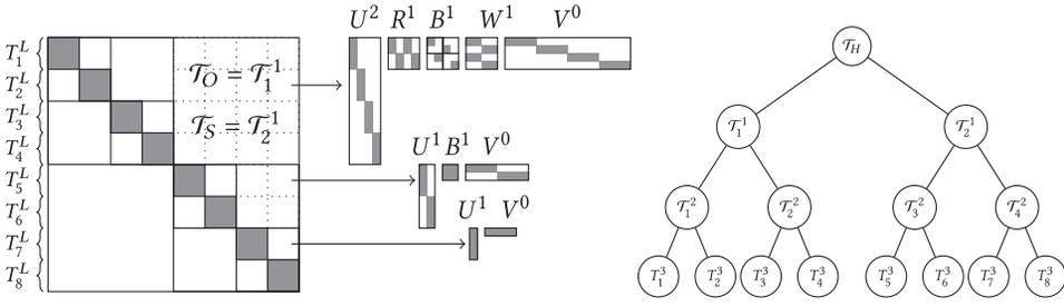
Fig. 4. Illustration of a four-level hierarchically off-diagonal butterfly matrix. The root node is at level  $l = 0$ , and all leaf nodes are at level  $L = 3$ . The two largest off-diagonal blocks are approximated using two-level butterfly matrices. The four off-diagonal blocks one level down in the hierarchy are approximated using a one-level butterfly ( $U^1 B^1 V^0$ ). Finally, the smallest off-diagonal blocks are approximated as zero-level butterfly matrices.
