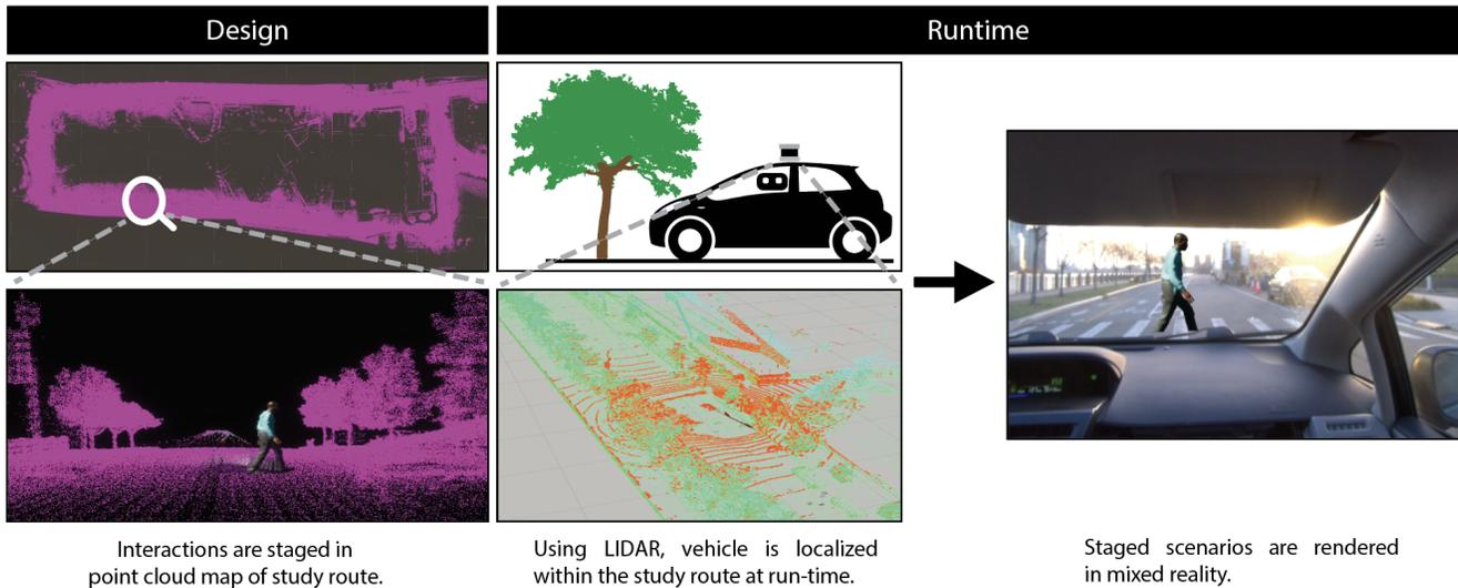
**Figure 2: Complete execution pipeline using the Portobello infrastructure. During the design phase, researchers can drag and drop virtual objects on the point cloud map. At run time, the LiDAR-based navigation system locates the vehicle’s position within the same map and sends the relative vehicle position to Unity. As a result, passengers wearing the video-see-through headset can see virtual objects at their corresponding real-world locations.**
