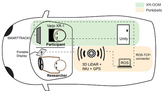
**Figure 3: The Portobello system uses a LiDAR-based navigation stack to localize the vehicle’s runtime position within a given map. The location information is transmitted to the Unity Desktop through ROS. The black dotted line indicates a virtual divider appearing only in the headset.**
