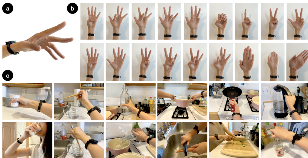
Figure 1: EchoWrist is a wristband that can understand 3D hand poses as well as hand-object interactions. (a) The EchoWrist prototype worn by a user. EchoWrist adopts a minimally-obtrusive design that keeps the device compact and low-profile. EchoWrist is able to (b) continuously track hand poses and (c) recognize various hand-object interactions.
