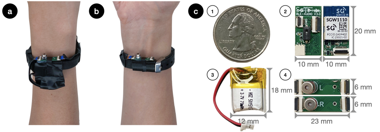
Figure 4: Hardware of EchoWrist. (a) (b) Wearing EchoWrist at the wrist. All components are mounted on a silicone wristband. (c) Customized PCBs for the microcontroller module and the sensing module. (1) US Quarter Dollar coin. (2) Customized PCB with SGW1110 module (front and back views). (3) 3.7 V 70 mAh LiPo battery. (4) Sensor module with speaker and microphone.
