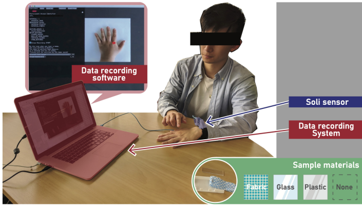
Fig. 9. The data collection setup for Study 2. A participant wears the Soli sensor device facing towards their left hand on their left wrist and performs gestures that is prompted on the laptop computer screen.
