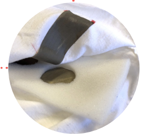
The initial button was made by gluing conductive woven ripstop on two fabric pieces separated with a 4 mm thick foam spacer with holes.
