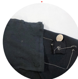
A hand-sewn soft circuit, powered with a 3V coin battery, inside of a T-shirt sleeve.
