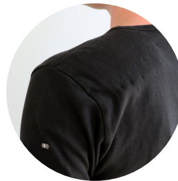
The final button was hand-sewn into a T-shirt with hidden stitches. An LED light was sewn to the sleeve and to the circuit to show a successful activation to the user.
