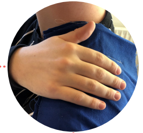
The best place to activate a soft button with a relaxed arm was found to be on the back side of the shoulder.
