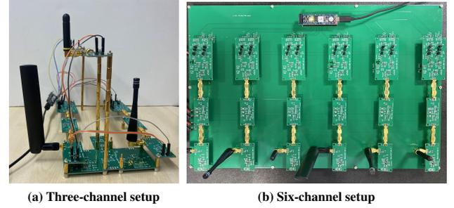
Figure 16: Different NEURORADAR configurations for (a) gesture recognition, and (b) localization.
