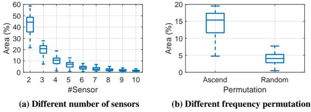
Figure 5: Localization ambiguity area with different settings.
