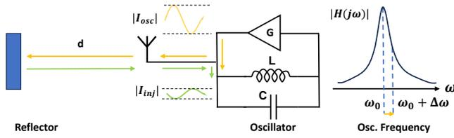
Figure 2: Self-injection locking.
