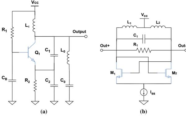
Figure 10: (a) Clapp oscillator, (b) cross-coupled oscillator.
