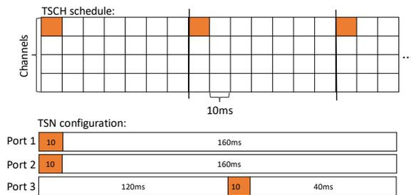
**Figure 2:** In the TSCH schedule (top), all the nodes use the colored cell for transmitting data/control packets. For the TSN schedule (bottom), the ports 1 and 2 (connected to the gateways) are open during the period [0-10]ms and port 3 (connected to end station) opens 120ms later for 10ms.
