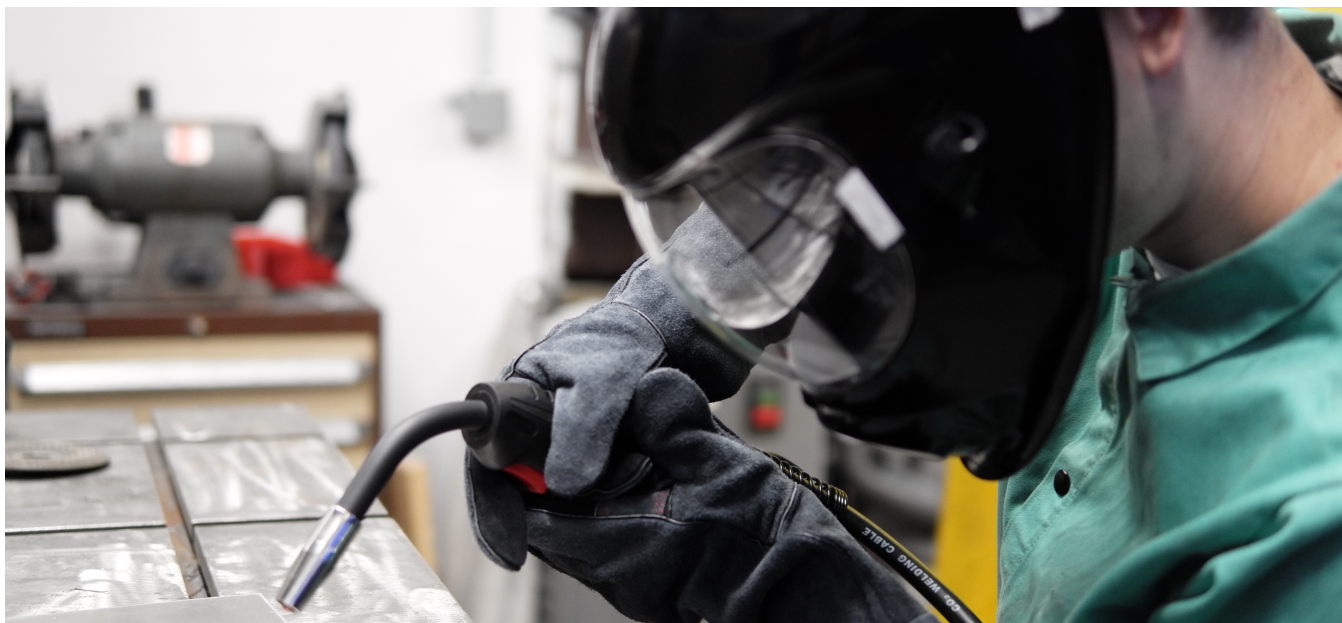
Figure 1: Integrated XR welding helmet and torch system.
