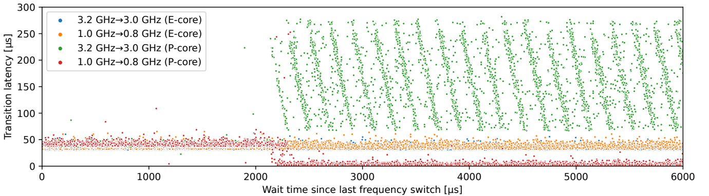
Figure 2: The time until a new frequency is applied depends on the wait time since the last frequency change. The latency for E-cores is independent of that wait time. Latencies on P-cores behave identical to those of E-cores for low wait times. For longer wait times, patterns emerge for P-cores which depend on the start and target frequencies.
