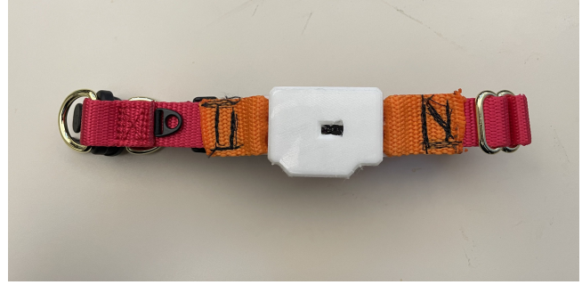
Figure 1: The activity monitor collar with sensors, microcontroller, and battery inside of the 3D TPU printed enclosure.
